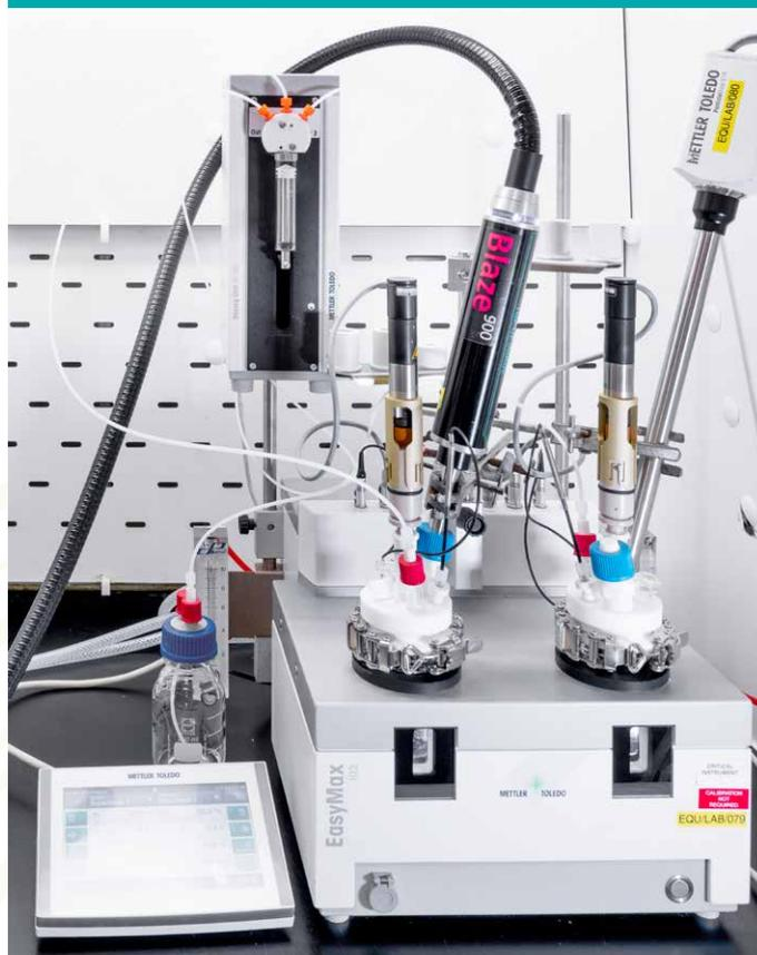
Process Analytical Tools (PAT) allow in-situ monitoring of crystallization.
