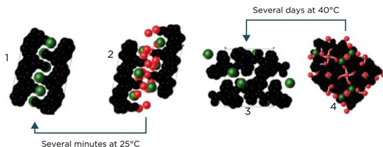
Initial data indicated that there were two anhydrous and two hydrated forms with the same amount of water observed in the two hydrated forms. Only detailed analysis by XRPD, single-crystal X-ray diffraction, DVS and thermal analysis showed that they were not true polymorphs of each other. This understanding then allowed the targeting of the desired form, selected on the basis of a variety of data.
