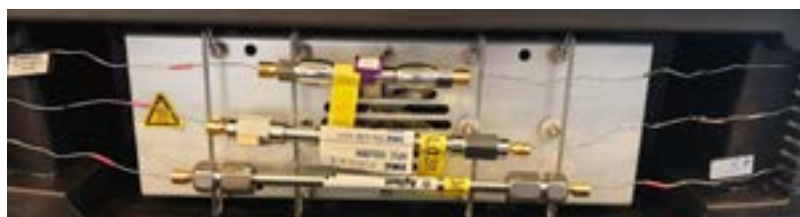
Common column screening setup utilizing 3 columns
