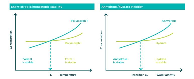
The phase boundary and stability window for each polymorph was determined experimentally using competitive slurries of various water activity media. The anhydrous polymorph was found to be stable at aw<80% and was selected for scale-up.
