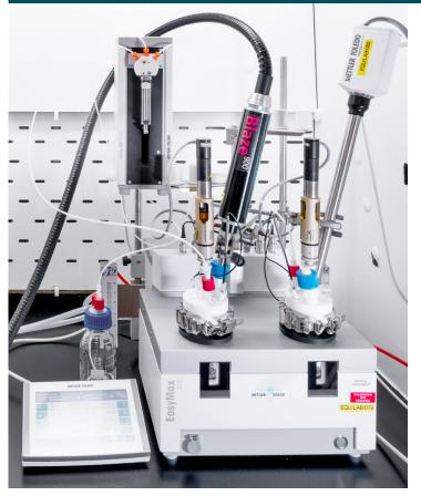
Process Analytical Tools (PAT) allow in-situ monitoring of crystallization.
